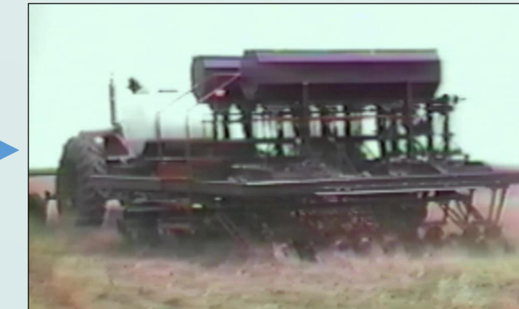
SDSU: Redfield/Dakota Lakes No-Till Drill Precision Placement and Controlled Traffic Beginning Step of Field Grid Sense and FGS Precision Farming Monitor
