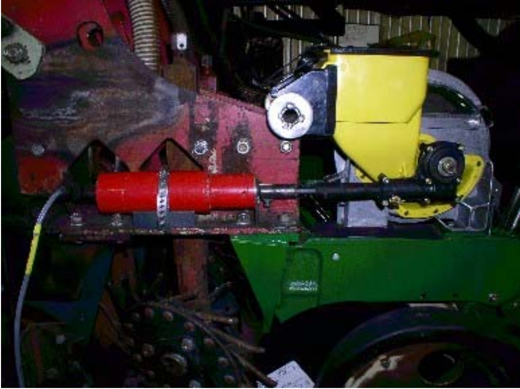
Dunkenmotoren electric drive attached to a standard JD vacuum seed meter.
